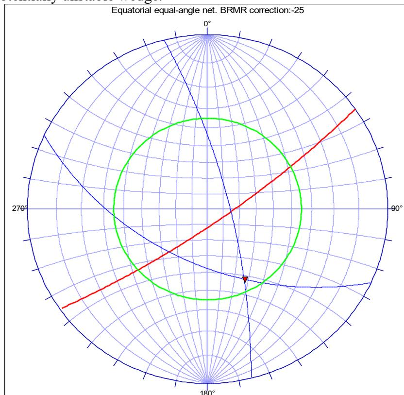
This condition happens when the wedge is oriented in the slope direction and the angle of shear strength is lesser than the angle of dip of the sliding line.
