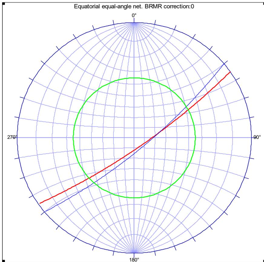
This condition happens when the slope and one of the discontinuity are approximately vertical and have a similar dip direction.
