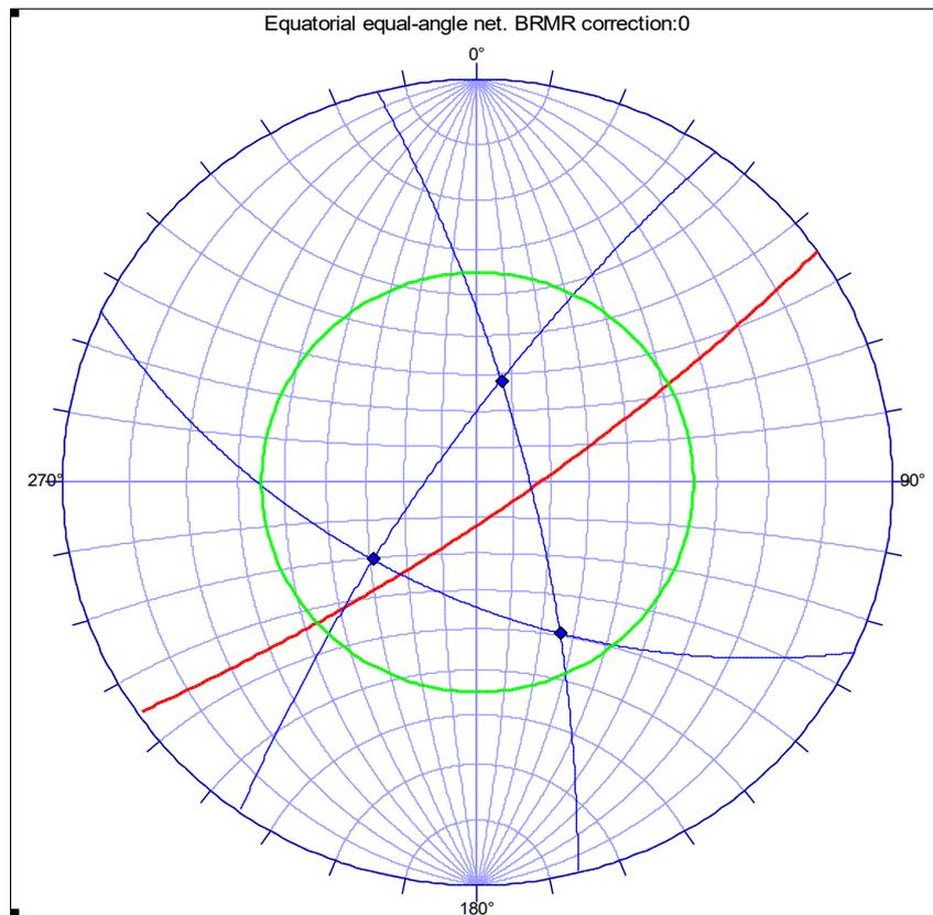
The presence of unstable blocks in the roof of a tunnel is put in evidence by the intersection of three or more discontinuities which form a closed shape.
