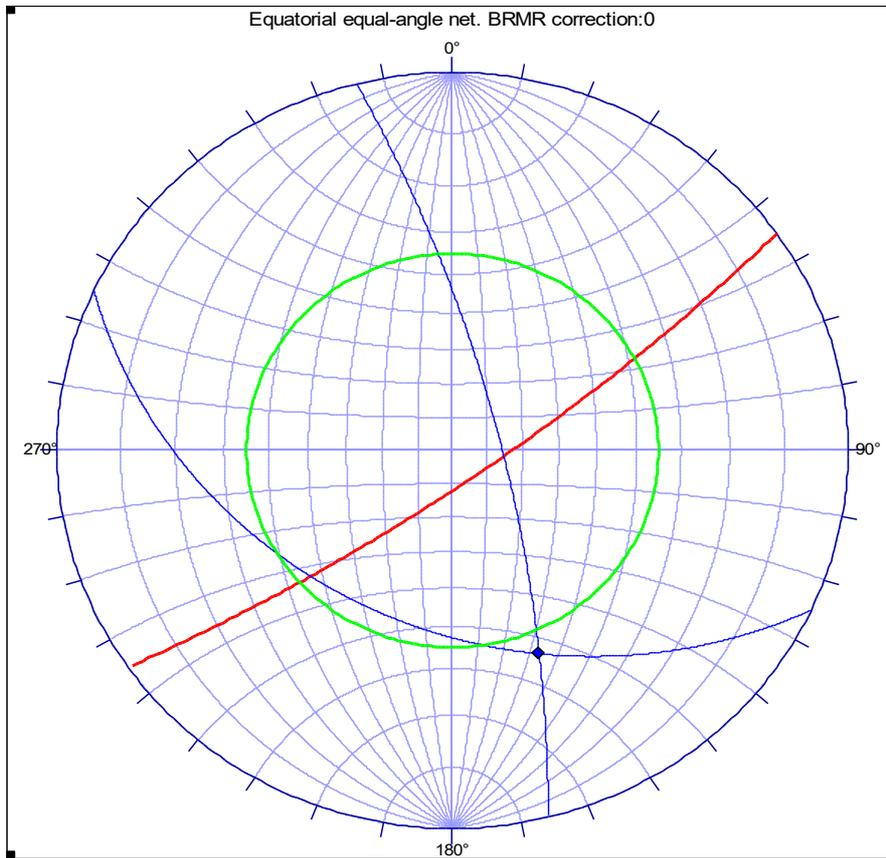
This condition happens when the wedge is oriented in the slope direction and the angle of shear strength is greater than the angle of dip of the sliding line or when the wedge is anti-dip slope oriented.
