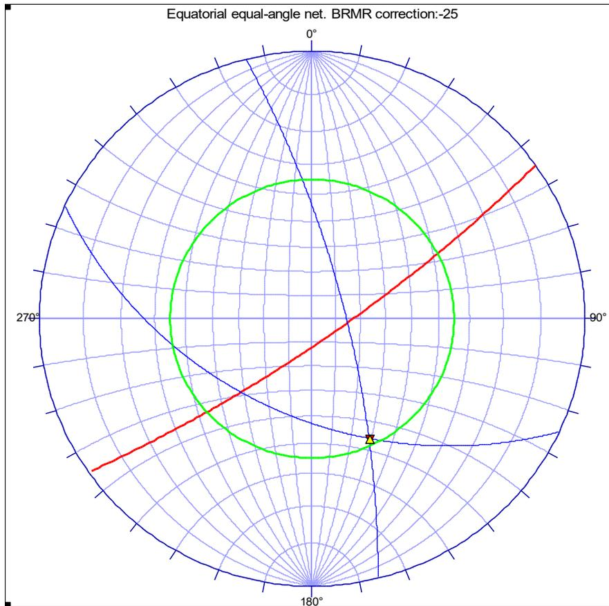
This condition happens when the wedge is oriented in the slope direction and the angle of shear strength is approximately equal to the angle of dip of the sliding line ( $\pm 2^\circ$ ).
